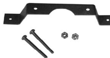
HMO-4517 Front mounting bracket for MEP-1200 series actuators (for use when actuator must be mounted remote of the damper shaft)—includes hardware to mount bracket to actuator
