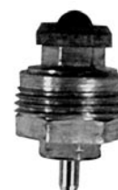
Bonnet Assembly (consists of stem, plug, packing, bonnet and disc): HPO-5030 1/2" 2.0 Cv, 2-way HPO-5031 1/2" 2.6 Cv, 2-way HPO-5032 3/4" 2.9 Cv, 2-way HPO-5033 3/4" 4.7 Cv, 2-way HPO-5034 1/2" 1.7 Cv, 3-way HPO-5035 1/2" 1.6 Cv, 2-way
