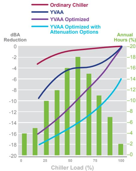
An optimized YVAA chiller can reduce ambient noise by as much as 16 dBA.
