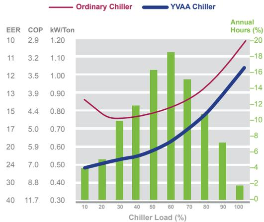
The YVAA chiller features the industry's lowest kW/Ton at both design and off-design conditions.
